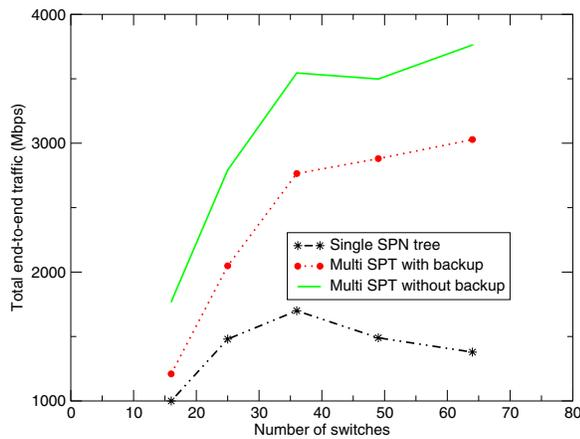
Fig. 5. Total end-to-end traffic in network with single spanning tree, and multiple spanning trees with and without backup provisioning. The network follows a uniform traffic pattern while communicating with each other.
