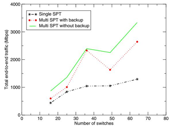
Fig. 6. Total end-to-end traffic in network with single spanning tree, and multiple spanning trees with and without backup provisioning. The network follows a skewed traffic pattern while communicating with each other. The case with 49 switches shows a dip in performance because of saturation of links near servers.
