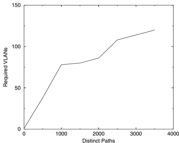
Fig. 8. The number of required VLANs with different number of paths. The required number generally increases with increase in number of paths.
