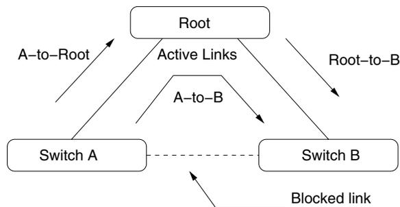
Fig. 1. Load imbalance scenario in single spanning tree. Three different flows, A-to-B, A-to-Root, and Root-to-B share same set of links despite the presence of a link between switch A and B. If somehow link A-B is made active, the overall network throughput can be improved significantly.
