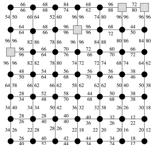
Fig. 7. Load distribution in a 7x7 grid network. The edges represent duplex links of 100 Mbps capacity. The links are marked with the total provisioned bandwidth. Note that certain links in the vicinity of servers (marked as squares) are completely saturated. This network can be tuned by adding new links in parallel to the existing links.
