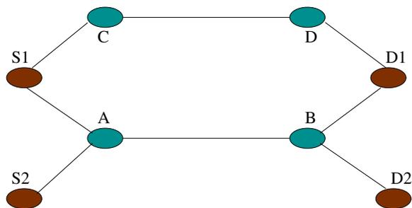
Fig. 2. A simple problem of selecting a route from  $S_1$  to  $D_1$ . Selecting the route  $(S_1, C, D, D_1)$  leaves the critical link  $(A, B)$  free for future virtual connections between  $S_2$  and  $D_2$ .
