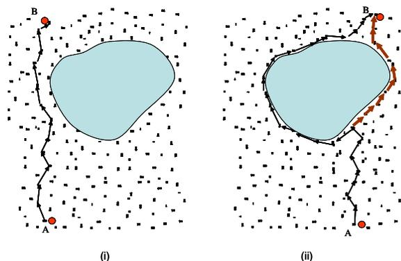
**Fig. 17.** A path migration scenario: (i) a multi-hop communication path is established between two mobile agents  $A$  and  $B$ , using the sensor network; (ii) as both agents move to the right, the path, shown as the thin line, gets stuck at the boundary of the hole. The improved path is shown as the bold line.
