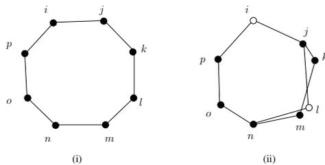
**Fig. 13.** Illustrations on cases for suppressed start: (i) the most common case in which suppressed start can effectively reduce traffic overhead; (ii) the case in which suppressed start may be overly suppressing, so that the hole belonging to node  $k$  may never get discovered as its messenger packet may get dropped by node such as  $o$ ,  $p$  or  $i$ .
