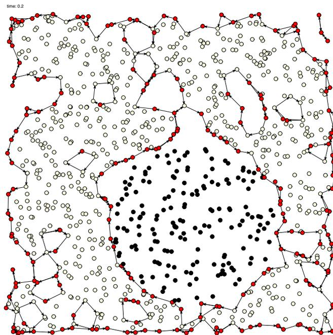
**Fig. 1.** The sensors in black failed, leaving a large “hole” in a network with sensors randomly placed. There are also small “holes” due to low sensor density. Small circles represent sensor nodes. Black nodes represent failed sensors. Red nodes represent stuck nodes that will be explained later.
